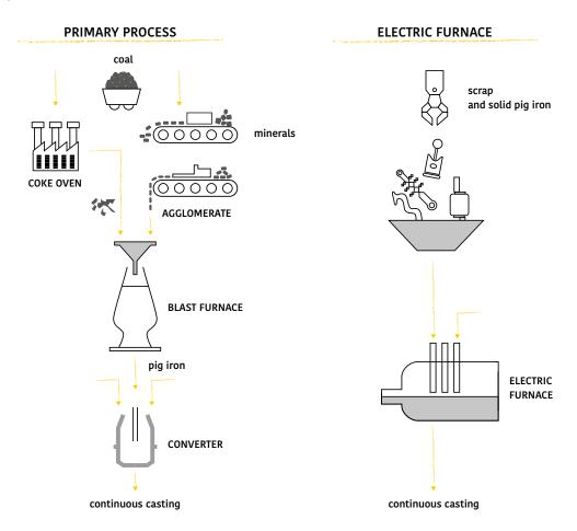
In the case of steel produced using the primary process, raw materials are prepared. In the agglomeration plant (minerals) and in the coke oven (coal) and then melted in the blast furnace forming liquid pig iron. The pig iron is passed on to the converters where, after the addition
