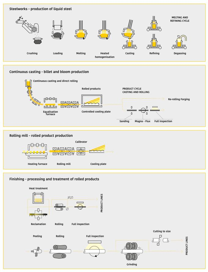
Acciaierie Venete's production starts with the electric furnace and is divided into the following steps:
